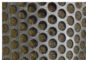
BEFORE EASYWATER SERIES C: Clogged Prefilter for Thermal Control Unit (Exterior View)
