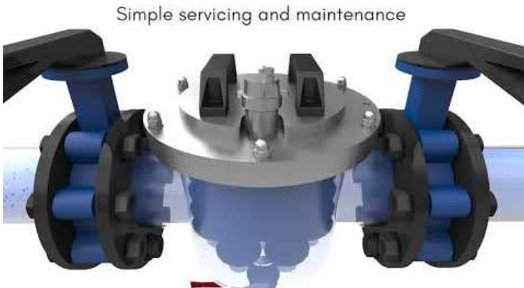
BoilerMagXT is a full-flow, single-pass insurance against metal in the system. It installs in the 1-1/2" to 12" heating or cooling system main. It is best installed on the return before the system pumps. It is most efficient if installed with 5 pipe diameters upstream. There should be service valves at the inlet and outlet.
