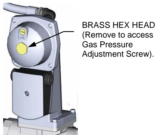
Figure 4-3: Gas Pressure Adjustment Screw Location
