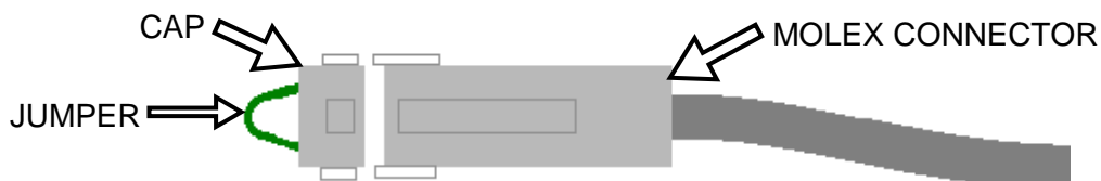
Figure 2-17: Sequencing Isolation Valve Molex Connector and Jumper Wire
