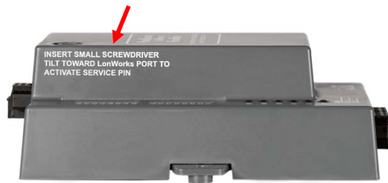
Figure 7-1: LonWorks Service Pin Location
