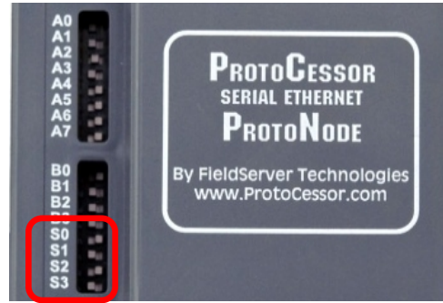
S Bank DIP Switch Location
