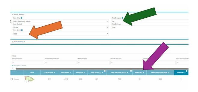
**Step 4**: Go back and change the speed to 1800 RPM and click "Get Results". The 4EB pump can do the future job at 25 HP so there is no change to the current pump. The extra 7% today or a few hundred dollars will avoid changing the pump, motor, and drive in the future.
