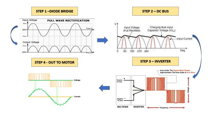
The drive takes the AC power, normally three-phase, and converts it to DC. We "flatten out spikes" so it looks like DC. Then it uses electronic transistors to invert it back to AC. When it changes it back to AC, the electronics change the voltage and phase. Phase is the width of the signal, and the height is the voltage. The variation of voltage and phase will change the speed of the motor.
