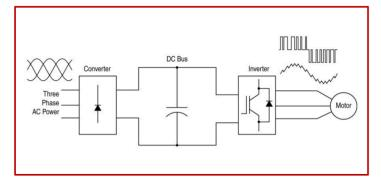
A HVAC variable speed drive (VFD) is an electronic device mounted in an enclosure which functions to change the speed that the motor is operating. The most prevalent type of VFD used in HVAC and plumbing is the pulse width modulated (PWM) type. Decades ago, two other early contenders were variable voltage and variable current types. These went by the wayside due to costs and ill effects on other system components. As an example, you may remember the tales of school clocks running backwards.
