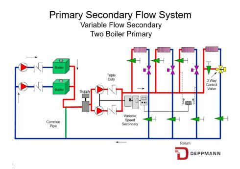
Remember, I said not to assume what one person is calling the loops. We will call the boiler loop the primary. The coil or system loop will be called the secondary. The pumps will have a head based on the very short piping to and from the boilers, the fittings, the check/balance valve, the common pipe, and the boilers. Fire tube boilers have rather small pressure drops compared with water tube boilers. In this case the pressure drop at 34 GPM is only 3 feet.
