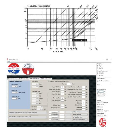
In our example, what if I used 2" copper pipe and made the common pipe 60 feet long and added two elbows and a ball valve to that pipe. Using the B&G system syzer, the answer shown is 1.68 feet. It will cause a difference, but not much difference.
