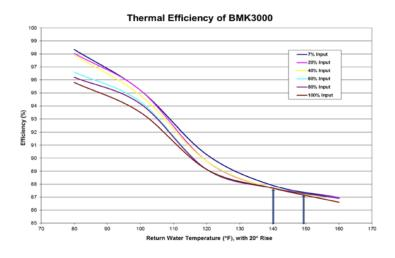
You can see that the published efficiency range of about 95.5% to 98% is at a cool 80°F. At a 140°F return temperature the efficiency at 100% load would be 87.8%. You could schedule the Benchmark and use the 87.8%. Unless the project documents were a base bid with mandatory alternates, you may end up with another brand. Will that brand have a true 87.8% at the design return temperature? Probably not.
