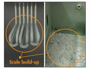
DriSteem Vapormist® humidifier heaters and tank after 90 days of intermittent runtime at 50% demand
