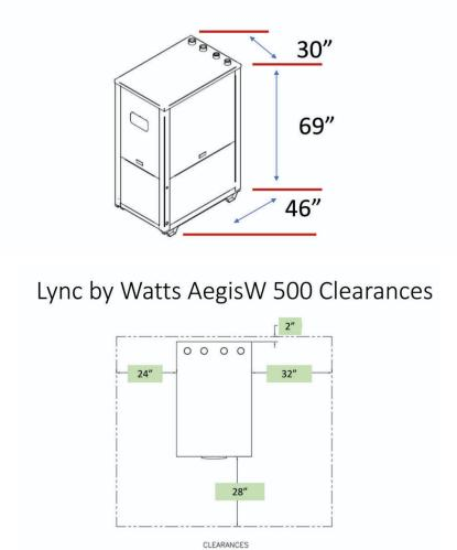
This heat pump is designed using the preferred R-744 natural refrigerant with a global warming potential (GWP) of 1.0 and an ozone depletion potential of 0.0. The use of this refrigerant will also allow a resetting of the outlet temperature to 160°F for any Legionella disinfecting processes.
