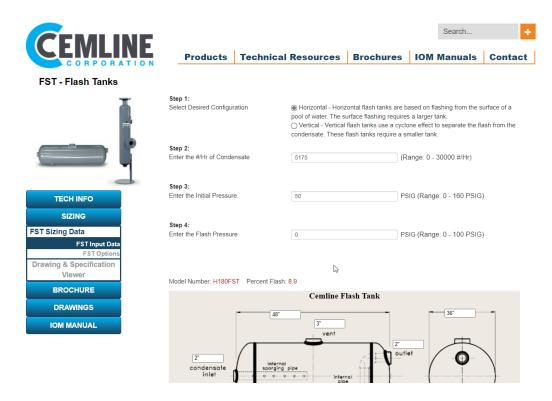
Notice the "percent flash" shown is 8.9%. That means that as much as 460 PPH (5175  $\times$  0.089 = 460.58) of flash steam at 0 PSIG could be lost up the vent of the flash tank. This is what the owner experienced once the flash tank was installed. The condensate unit was now protected but there was still flash steam now coming out of the flash tank.
