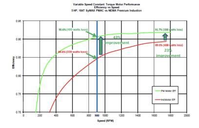
At the full 1765 RPM pump speed, the PMAC motor has a 23% improvement over the premium efficiency motor. When the motor is running at 50% speed, that efficiency improvement becomes 43%!
