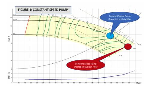
Figure 1 shows a constant speed pump. The selection at worst case is the blue dot. It meets the standard suggestion of being less than 85% of the end of curve. When you look at the clean selection, the pump runs out on the curve. The operation is at or just past the last acceptable point of operation. This is a case where selecting a pump farther back on the curve would be a prudent choice.
