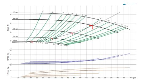
The impeller now becomes 9.25". The operating point will be 650 GPM at 55 feet with a brake horsepower of 10.6 at 1606 RPM. The operating point efficiency is 85.3%.
