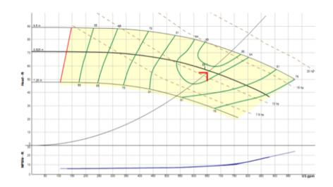
The exact operating point will be 650 GPM at 55 feet with a brake horsepower of 11 at 1770 RPM full motor speed. The operating point efficiency is 84.7% and a 8.625" impeller is required.
