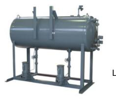
Last week, we described the <u>operation and key selection criteria for a condensate return or</u> <u>transfer unit</u>. The important operational characteristic of a transfer unit is the pump operation is a result of a float in the receiver of the unit itself. The goal is to recognize there is condensate in the receiver and pump it out quickly.
