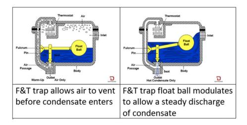
The thermostatic portion of a F&T steam trap allows for fast venting. The float ball allows for modulation of the amount of condensate leaving the trap. There is no need to prime the trap for proper operation. The trap will operate at very low loads without any issues.
