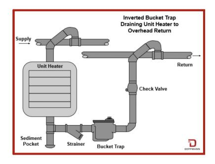
The trap would be a Hoffman series B0 with a maximum pressure of 20 PSIG and 450 PPH at a 5 PSIG differential across the trap. Since the trap does not modulate, it will always provide 5 PSIG drop at 450 PPH.
