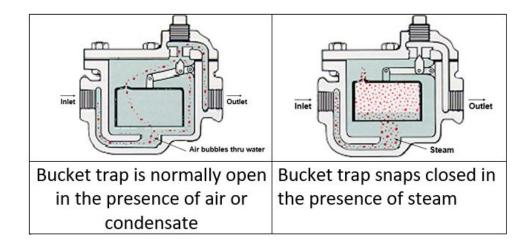
Bucket traps are on-off style. They are sized for a given pressure drop at the rated flow rate.
