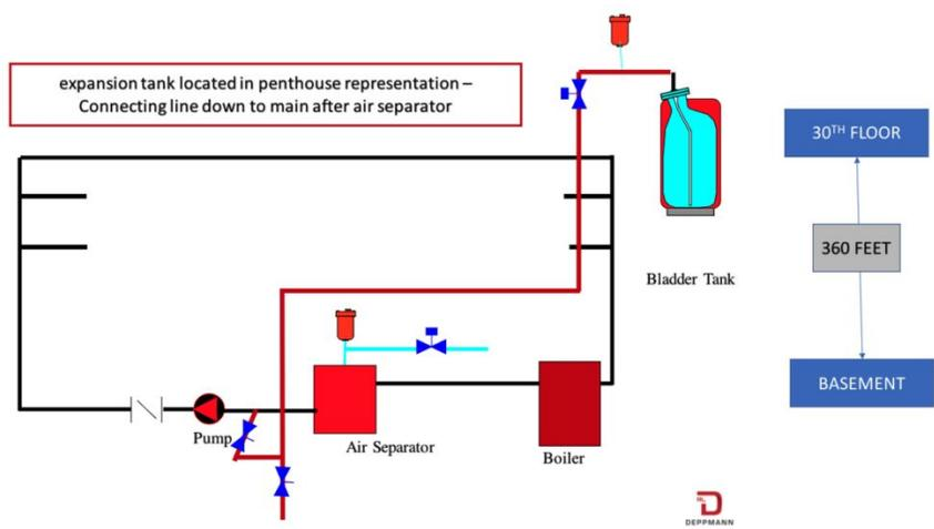
In this system example, we show the tank mounted in the penthouse and the connection in the basement. The point of no pressure change is after the air separator and before the pump. One big advantage
