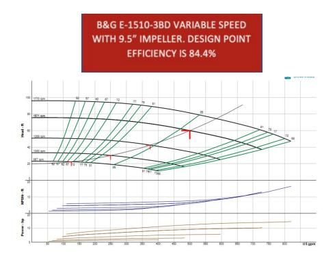
If we use the 9.5" full-sized impeller and adjust the speed down to 1571 RPM, the pump will give the design flow and head, but the efficiency is now 84.4%. This is an increase of 2.0% over the trimmed impeller. The pump is non-overloading with the 15 HP motor at both full speed and the 1571 design speed. Seems like this is a win-win in this example.
