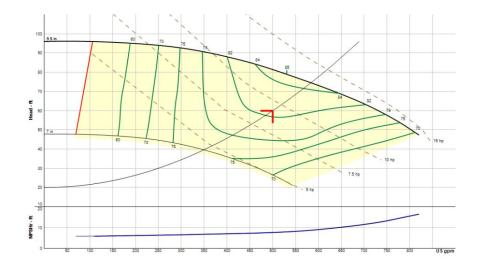
Here is a constant speed curve for a e-1510-3BD from the <u>Bell & Gossett ESP-Systemwize</u> selection program. Notice at the full runner 9.5" impeller there is a point, the best efficiency
