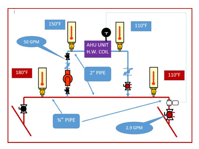
What are the pros and cons of this change? Well, the only negative is the additional cost of the coil. I called our friends at the Trane Company and asked for the impact. The 180°F coil will be a series D3WB with 2 rows. The 150°F coil is a DW0B with 3 rows. If there were 4 of these air handling units, the cost impact will be about \$3,000 each or \$12,000 total additional first cost. Why spend \$12,000 more?
