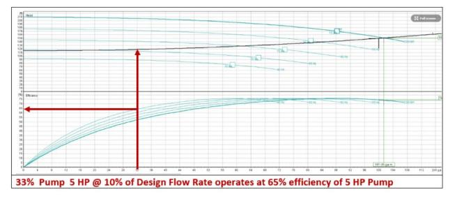
What you may notice is the larger pump is using more horsepower at lower efficiencies. The smaller pump is using less horsepower at higher efficiencies. Using the flow profile for our example problem and staging the smaller pumps will result in less energy use. Here is the table showing the energy consumed. I looked at our example 300 GPM system and a larger 600 GPM system.
