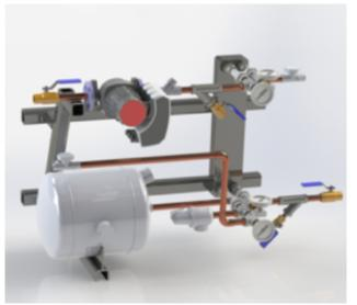
individual zones to drop the pressure below the 80 PSIG limit. These PRVs may be installed with the required hot water recirculation design and equipment or you may use a packaged <u>high rise recirculation package</u>. The key point here is the words "*all of the water*". Only part of the water goes through the PRV. The part in the zone the PRV services.
