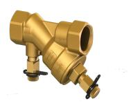
These valves will self-adjust to maintain the flow rate. They do not require the plumbing contractor to set the valve and the owner cannot open them later in the life of the system. For these reasons I deem this to be a "BETTER" solution. This type of balance is also constant flow so energy will be wasted.
