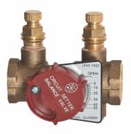
This balance valve allows the plumbing contractor to have the system balanced by throttling the valve. The ports provided allows reading out the pressure drop and referring to programs or tools to determine the flow rate during and after adjusting the valve. A memory stop assures the valve will be returned to the correct setting if the valve is used for its 100% shutoff capability during service.
