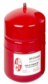
The B&G HFT tank is a non-code small diaphragm tank with a maximum of 100 PSIG working pressure. This tank is used where ASME is not required and the system is a lower system volume. An example is a residential system.
