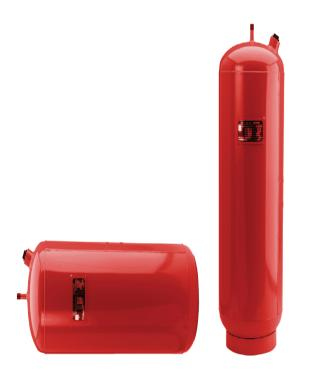
The "D" style tank is an ASME diaphragm tank. The cost is significantly lower than a "B" or "B-LA" tank. The diaphragm is not replaceable so you must make sure the tank can be removed if it needs to be replaced. This tank is a great option when you find your selection is one of the smaller tanks. This tank may be physically smaller than the "B" choice and at a lower price point.
