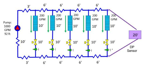
Here is a simple system with 6 zones. To make things easier to see, I made the design flow rates all the same. Each zone could be several terminal units, a single air handling unit, or an entire floor of a larger building. Long before the balancing contractor arrives to throttle the balance valves, Mother Nature will use physics to balance this system. What does this system look like before it is balanced? Let's use an example system to see what this looks like.
