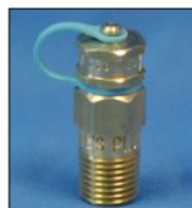
Product: #100 Core: Neoprene Thread: 1/4" NPT Length: 1 1/2"
