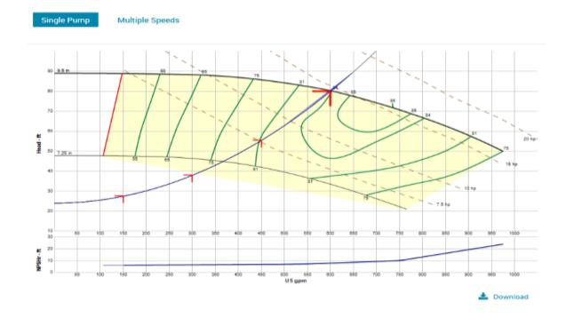
The design point is 600 GPM at 1770 RPM, 80 feet of head at 1770 RPM, and 14.5 brake horsepower at 1770 RPM. What do these numbers look like at 1858 RPM or 5% more speed?
