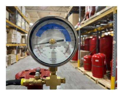
One differential pressure gauge, installed using the same taps at the pump inlet and outlet, can eliminate the problems noted above. Note that the gauge kit will need to be installed properly on the pump suction and the pump discharge ports to ensure the readings are usable. By eliminating the use of two gauges, the rate of error will drop to the accuracy rating for the single pressure gauge.
