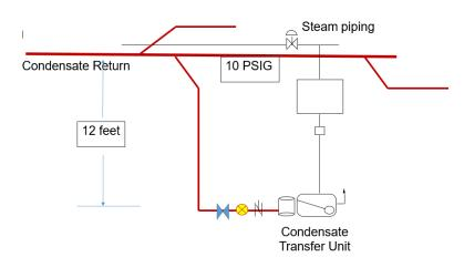
5 PSIG. The pump will be selected for 90 GPM at 26 PSIG or 63 feet. Most condensate pump selections would round the number up to the nearest 5 PSIG but will assume the head is 63 feet.
