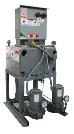
Pump seal limitations for condensate pumps such as the Domestic CC, CB, and CBE style units rated for 250°F. Since the receiver is vented, there is no concern about seal temperature for these Domestic models. The second concern is the pressure available at the pump suction to keep this high temperature water from flashing into steam. In general, the condensate pumps must have a low NPSHR (net positive suction head required) to handle the low pressure higher temperature condensate.
