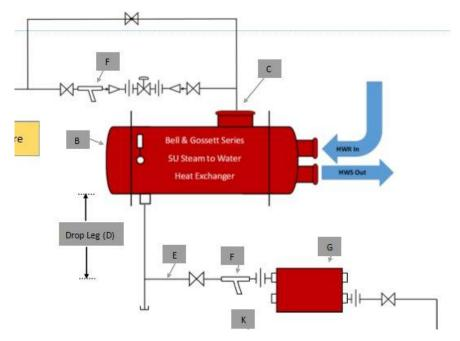
Normally, strainers are placed before control valves on the steam side of the system, and before traps and condensate pumps on the condensate side of the system.
