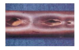
the tube bundle. The image below shows damage to a tube caused by water hammer.
