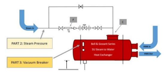
Vacuum breakers should always be used on steam-to-water heat exchangers. They prevent condensate from being held up in the shell, which can lead to water hammer and tube damage.
