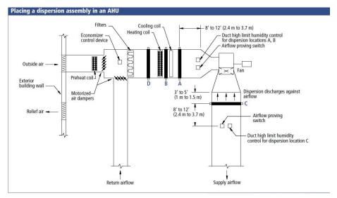
As a third choice, we could look at location C if there is adequate space to install the dispersion assembly. But we would have to be careful of turbulent flow, which could impact the steam absorption distance. All three of these locations occur after the heating coil, so the air is at its warmest. Point D would be a poor location do it because of the cold air stream.
