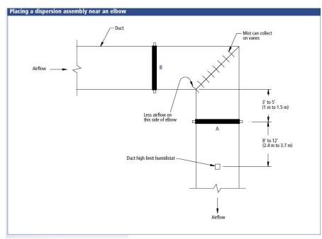
In this scenario, location A is the best choice. This is because better absorption occurs downstream of the elbow. If there isn't enough straight duct at this location, then B can be considered—but we must be careful to not wet the turning vanes. If B is chosen, we highly recommend installing a multiple tube unit to make sure you have complete absorption. In either case, it's best to discharge the steam against or perpendicular to the air stream to provide the best possible absorption.
