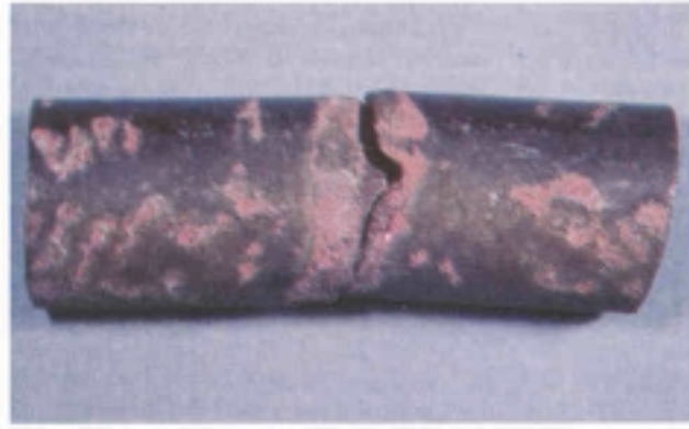
Fig. 20. Corrosion-fatigue attack on tube.
