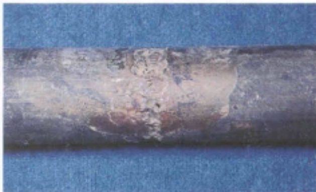
Fig, 17. Crevice corrosion at contact between tube and baffle. Fig.18. Condensate grooving and pitting attack on tube.
