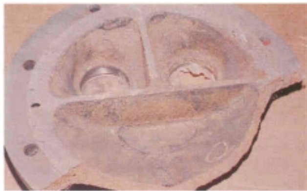
Fig 8. Thermal expansion failure of cast iron head.
