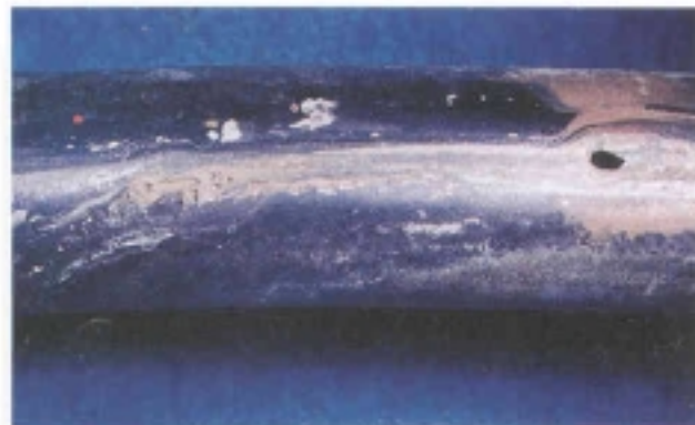
Fig, 17. Crevice corrosion at contact between tube and baffle. Fig.18. Condensate grooving and pitting attack on tube.
