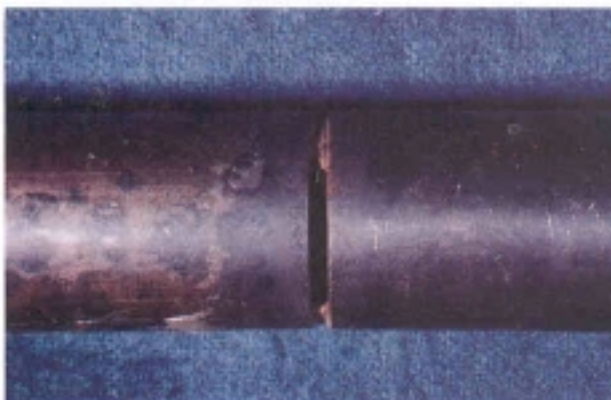
Fig. 4. Velocity-induced vibration cut of tube.
