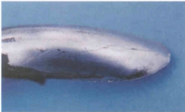
Fig 13. Carbon dioxide pitting attack on copper tube.
