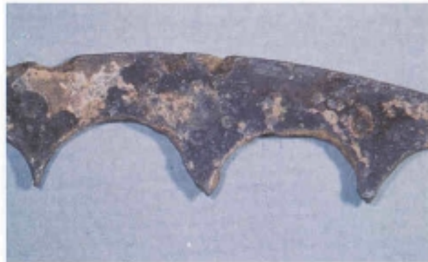
Fig. 14. Stress corrosion failure in admiralty tube.
