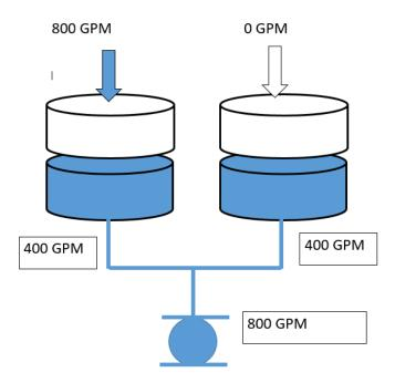
pump will air lock and stop pumping. Meanwhile, the tower in operation overflows.
