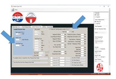
suction piping pressure drop. I found a note in a BAC tower article reminding the engineer not to forget the entrance and exit pressure drop. It added about 40 feet of TEL! Thank you BAC—I won't forget it in the future.
