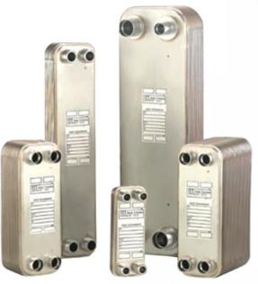
heat exchangers assume equal flow in each channel. To avoid flow maldistribution, Bell & Gossett recommends a maximum pressure drop through the nozzles less than or equal to 40% of the total pressure drop of the heat exchanger. For example: If the total pressure drop is specified to be 15 PSIG, the pressure drop for the entrance and exit nozzles should be less than 6 PSIG ( $15 \times 0.4 = 6$ ).
