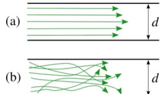
(a) Laminar flow (b) Turbulent flow
