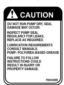
label indicates that the pump or frame is built with polyurea based grease. Morton Grove pumps or frames **WITHOUT** this new label were built before Dec 1<sup>st</sup> and have lithium based grease. The only exception is VSX Series pumps, which have always utilized polyurea based grease.
