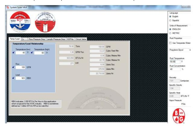
The first tab is marked **TEMP/LOAD** and in this example I entered temperatures of 40°F to 60°F as well as 100 GPM. Calculating the load for water is normally simple on a calculator. but in this case I changed the fluid to 30% propylene glycol/water.
