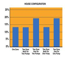
In general, there will be a 10% to 15% reduction of fuel usage in a house with a boiler that has a single circulating pump.
