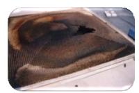
The second type of corrosion is "Local" corrosion which can be very harmful to a cooling system as shown above. The Wave allows system operation at mineral concentration levels above the saturation of calcium carbonate, thus providing the protection of a microscopic layer of CaCO3 as an effective natural corrosion inhibiter against "local" corrosion.
