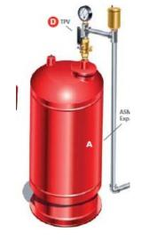
Diaphragm expansion tanks have a physical barrier inside the tank which acts to limit the expansion of the diaphragm. Bell and Gossett "D" style diaphragm tanks are ASME constructed and designed for either horizontal or vertical installation. The only difference is the location of the drain fitting. The "diaphragm" is limited in movement and, therefore, the acceptance volume is less than the tank volume. The separation between the air and water is mechanical.
