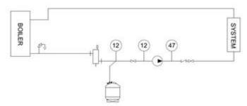
Using last week's article, we know the minimum cold fill pressure is 10.5 PSIG. Since the B&G B7-12 pressure regulating valve is factory set at 12 PSIG so let's be smart and set of cold fill pressure at 12 PSIG rather than 10.5.
