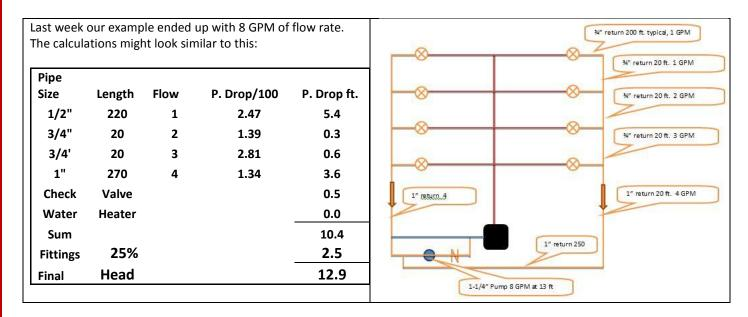
So our pump would be selected for 8 GPM at 13 feet. The Bell and Gossett ESP-PLUS program offers many solutions. We would select a B&G model PL-30B lead free bronze body pump with 1-1/4" flanges using a 1/12 HP, 115/60/1. We would also suggest the specification of the B&G CB-1/2LF lead free circuit setters for balance valves.
