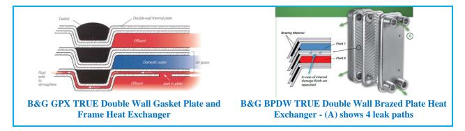
The Bell and Gossett double wall heat exchangers provide the protection of "TRUE" double wall construction, the air gaps required by code, and multiple leak paths for your peace of mind if any single leak path plugs.
