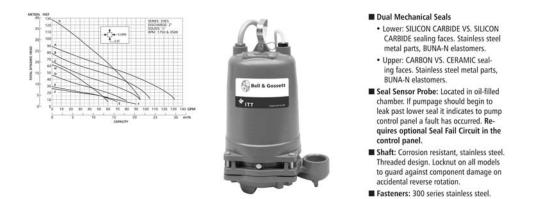
You want pump guide rails, and based on the <u>MMM article from 5-17-10</u>, you select the recommended 60" diameter sump for 3" pipe. Today's article advises you have 500 gallons of storage between pump on and off. Based on the chart above, you will require about 42" of storage level.
