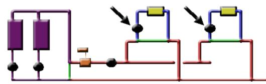
In our example above the purple piping is normally called the "Primary System". This is the system with the boilers and boiler circulating pumps.
