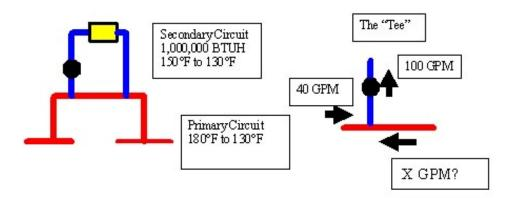
The law of the tee requires the flow rate into the tee to equal the flow rate out of the tee. If there is 40 GPM of 180° water coming in from the primary and 100 GPM of 150° water leaving the tee into the secondary, there must be 60 GPM of return water coming back into the tee from the secondary system return. This return water is 130°.
