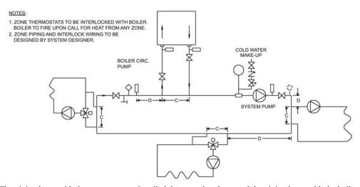
The piping loop, with the system pump, is called the secondary loop, and the piping loop, with the boiler, is called the primary loop. The three pumps, off of the secondary loop, would be referred to as tertiary loops.
