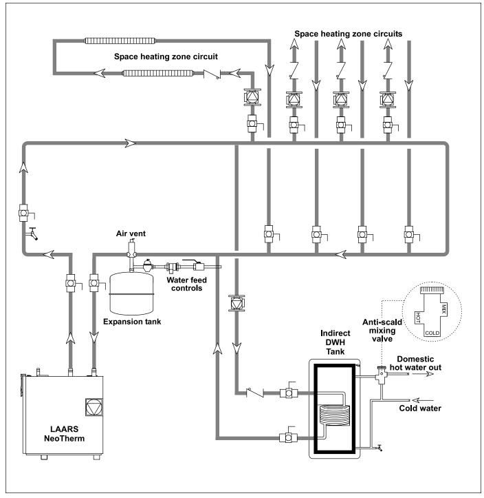
Figure 11. Hydronic Piping — Single Boiler with Indirect DWH Tank (zoning with circulators)..
