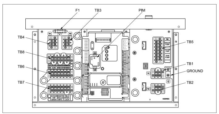
Figure 18. Control Panel Layout.
