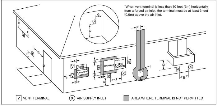
Figure 9. Combustion Air and Vent Through Side Wall.
