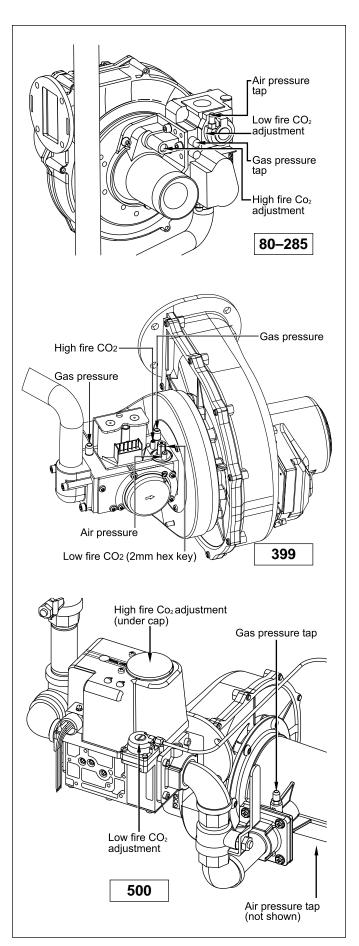
Figure 22. NeoTherm Gas Valves (285, 399 and 500).
