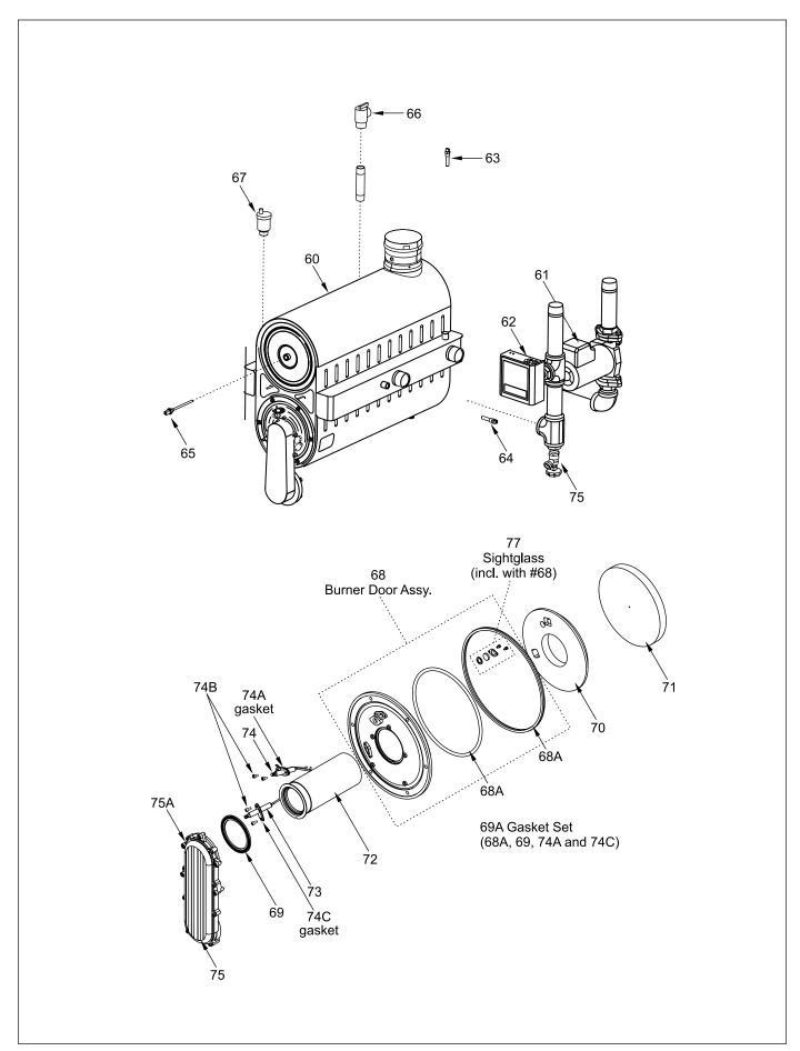
Figure 27. Heat Exchanger Components.
