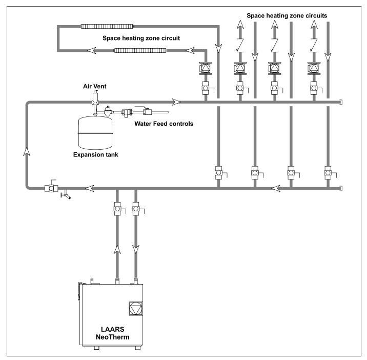
Figure 10. Hydronic Piping — Single Boiler (zoning with circulators).
