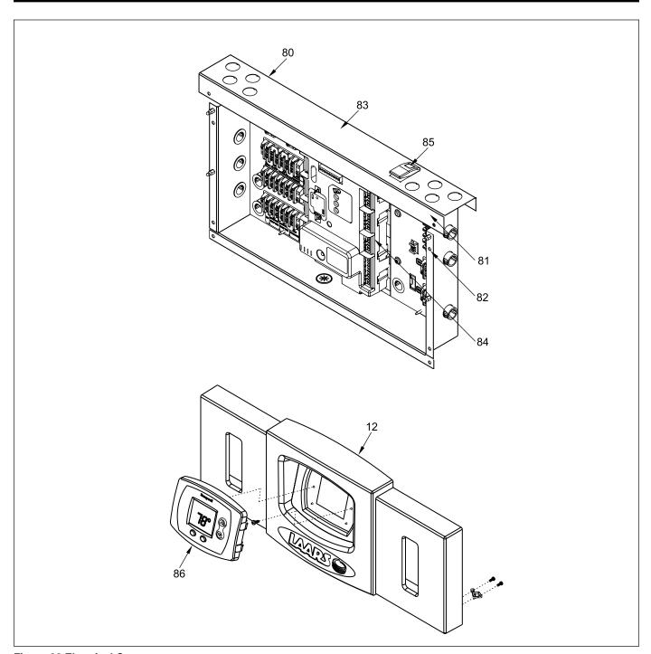
Figure 28 Electrical Components.
