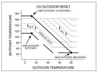
Figure 19. Outdoor Reset Setpoint Temperatures.
