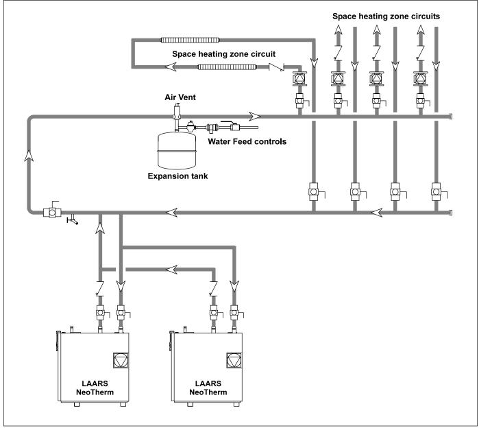
Figure 13. Hydronic Piping — Multiple Boilers (zoning with circulators).
