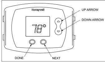
Figure 17. Control Buttons on User Interface.
