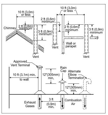
Figure 8. Combustion Air and Vent Through Roof.
