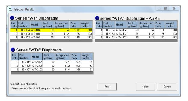
We could use a B&G WTA-404 ASME tank or one of the non-code choices. The ASME tank would have a 68-gallon volume with a maximum acceptance of 34 gallons and a drawdown of 3 gallons.
